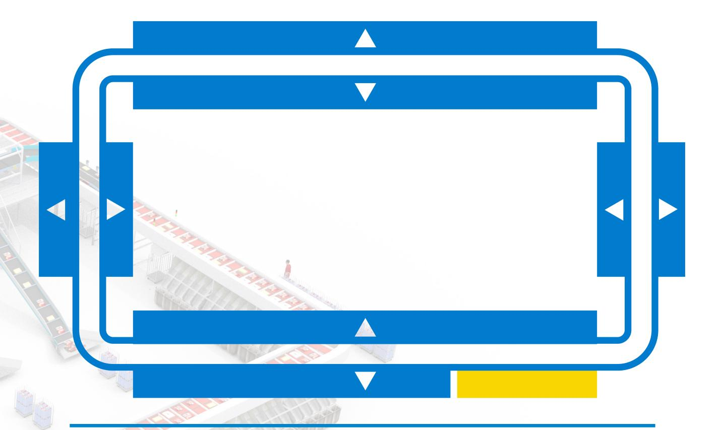
The extra wide oval layout is perfect for spaces that allow a square-like built. It maximises the amount of stations by placing them on all four sides. An optional automatic infeed can be placed in the center of the sorter.
