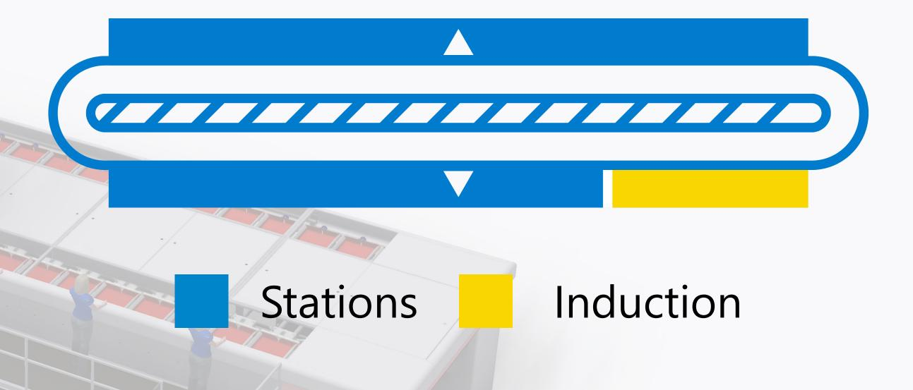
The closed oval layout enables a space saving solution. The height and width offers the most compact solution in the split tray sorter family.
