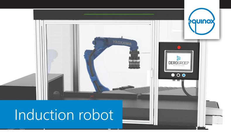
The induction robot picks items from bulk delivery and feeds it directly into a sorter. By automatically picking and placing items, your logistic process becomes more reliable and is able to run 24/7.
