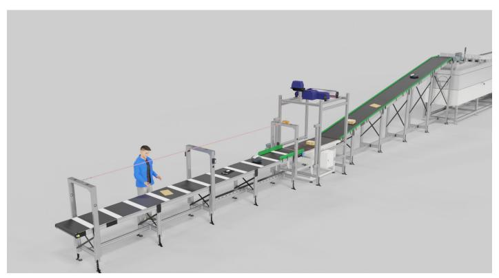
You can start with 1 robot cell at one side of the belt. The robot can induct 1.500, so 6.500 remains for 5 manual operators.
