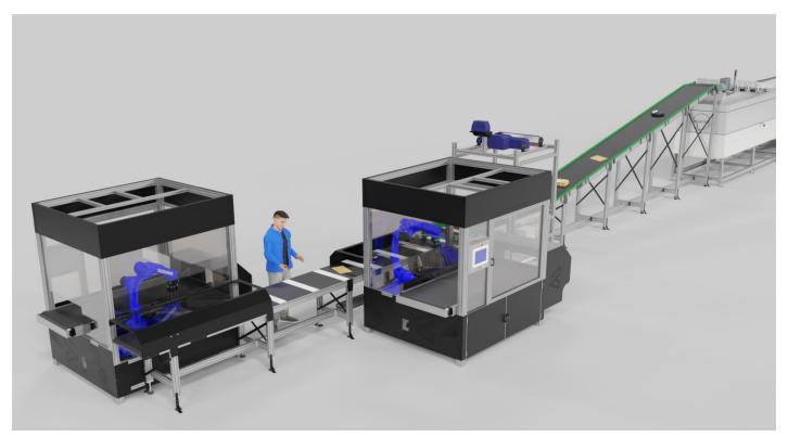
With 3 cells 8.000-3x1.500=3.500 remain for manual induction for 3 manual operators. And with 4 cells 8.000-4x1.500=2.000 for 2 manual inductors. This is the maximum you can automate as there will always be items not picked by the robot cells. The vision technique and deep learning database will continue to improve with less manual operation required in the near future.
