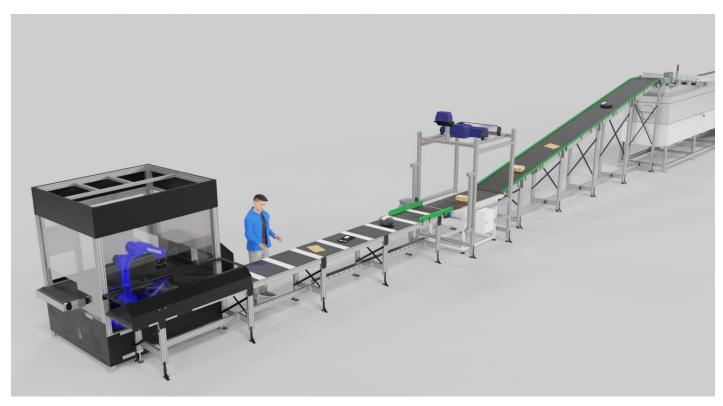
Items need to be inducted on the front, this can be done by emptying bags, boxes, roller cages into a hopper feeding the belt to the robot. Items not picked by the robot are collected in the box ate the rear of the cell. An operator inducts these parcels manually.
